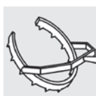
G-33757 FINE-THORNTON FIXATION RING for clear cornea and refractive procedures 16 mm diameter, 10 mm opening 12 atraumatic teeth, swivel handle
